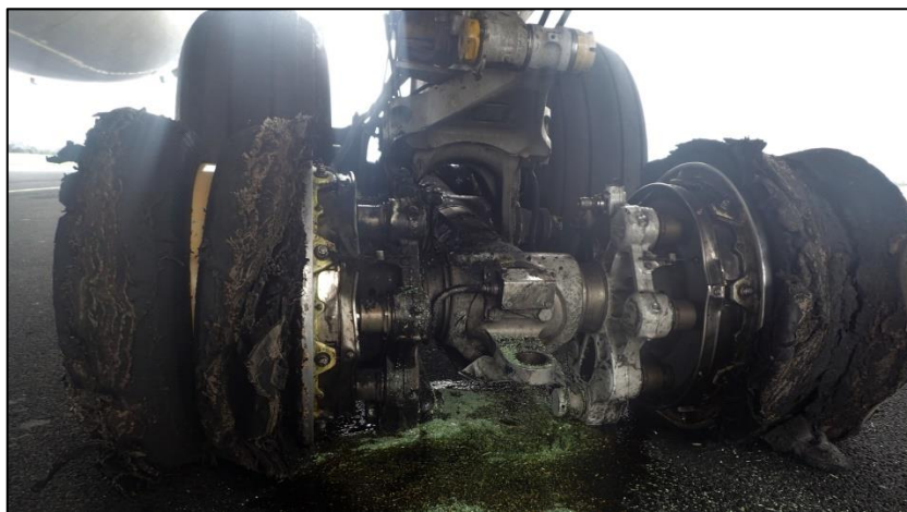
Photo No. 1: Fire Damage to Left Main Landing Gear (looking rearwards)
